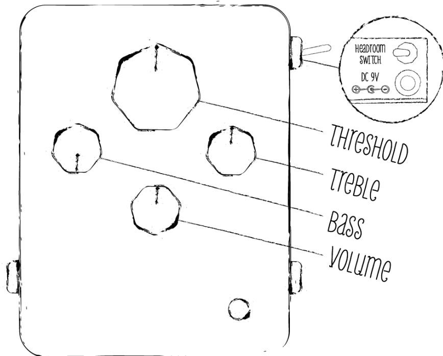
Marrakesh Preamp Console has four adjustment knobs:
