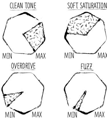
In Low Headroom mode, the pedal power is classic 9 volts. This is a typical power supply for guitar pedals. Low Headroom mode allows you to get more harmonic distortion of your signal, more hard compression and less output volume. Due to the limitation of the supply voltage, the overdrive becomes crumblier and is achieved much faster, saturation is also achieved quickly and becomes harder, fuzz at the minimum values of the Threshold knob is more "hairy" and clipped.
